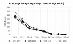
Fig. 1. BOD₅ change from inlet to outlet (High Temp, Low Flow, High BODin)
