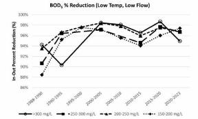
**Fig. 3.** Inlet to Outlet BOD<sub>5</sub> percent reduction from 1988 to present (Low Temp, Low Flow)
