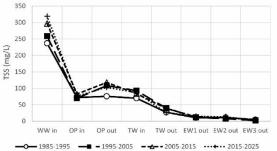
Fig. 2. TSS change from inlet to outlet (High Temp, Low Flow, High TSSin)
